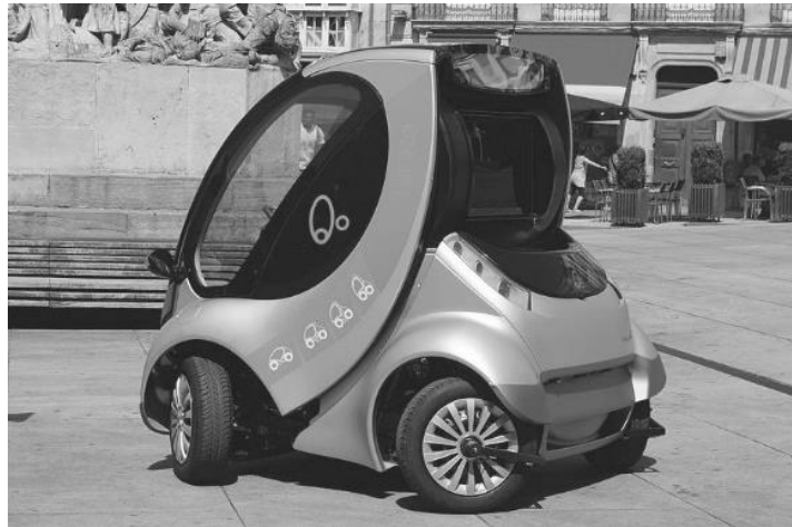
Figure 14. Hiriko Fold—a vehicle employing in-wheel motors.
