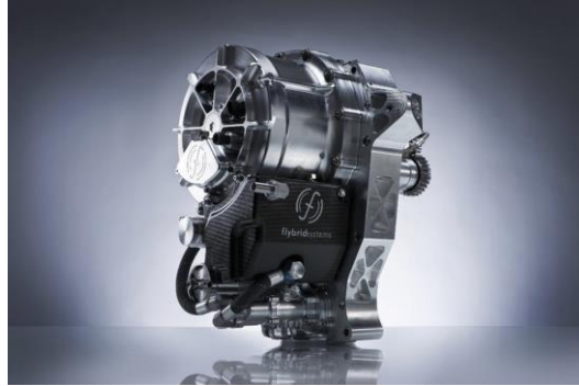
Figure 5.15 The Flybrid® hybrid system (Source: http://www.flybridsystems.com )
